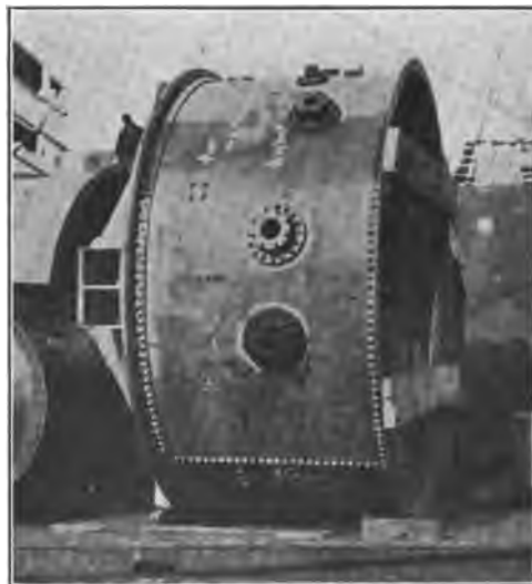
FIG. 142.—Another view of vacuum pan shown in Fig. 143, showing bracing.
